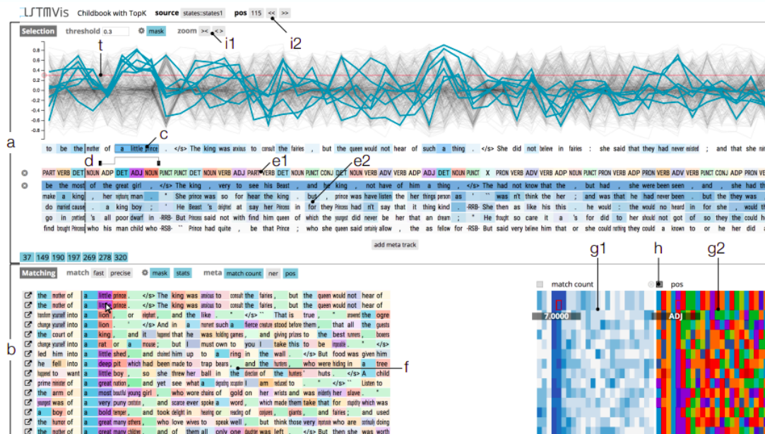
Fig. 1. The LSTMVis user interface. The user interactively selects a range of text specifying a hypothesis about the model in the Select View (a). This range is then used to match similar hidden state patterns displayed in the Match View (b). The selection is made by specifying a start-stop range in the text (c) and an activation threshold (t) which leads to a selection of hidden states (blue lines). The start-stop range can be further constrained using the pattern plot (d). The meta-tracks below depict extra information per word position like POS (e1) or the top K predictions (e2). The tool can then match this selection with similar hidden state patterns in the data set of varying lengths (f), providing insight into the representations learned by the model. The match view additionally includes user-defined meta-data encoded as heatmaps (g1,g2). The color of one heatmap (g2) can be mapped (h) to the word matrix (f) which allows the user to see patterns that lead to further refinement of the selection hypothesis. Navigation aids provide convenience ( i_1, i_2 ).
